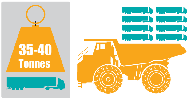
Load capacity of a Hitachi EH5000 dump truck is 320 tonnes.
