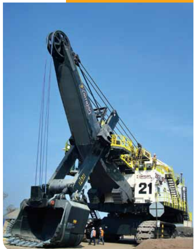
In 2011, Corrección's operation received 3 PH2800XPC shovels, each with a bucket capacity of 63.5 tonnes, equivalent in weight to 42 private automobiles.
